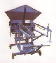
DIPTI Double Bucket scale type weigh Batcher having M.S. Fabricated buckets, each bucket capacity 220 Kgs. Division with towing accuracy + 2%, Scale fitted front side of the bucket., Quality fabrication, Steel wheel with towing arrangement for easy movement & Transportation. Tool box provided to keep weights are: 100Kg. 50Kg. 20Kg. Duration: length 1860mm. Height 1850mm width: 1290mm
